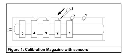
Using the diagram for guidance place the sensors so that they fit snugly into the magazine. Run the wires along the slot in the calibration magazine. Make sure that the channels are arranged in the order shown.
